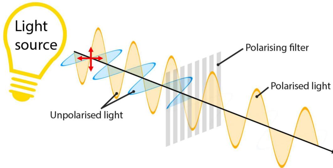
Vertical polarising filter blocks horizontally polarized photons and lets through vertically polarized photons
